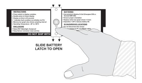
Use new, premium quality Alkaline D-Cell batteries only (Energizer E95 or Duracell/Procell MN1300).
