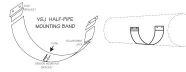
VSJ32-40 32-40" / 800-1000 mm ID pipes VSJ42-54 42-54" / 1100-1375 mm ID pipes VSJ56-72 56-72" / 1400-1800 mm ID pipes
