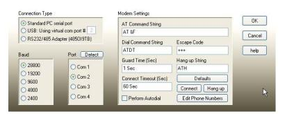
Stingray baud rate is fixed at 28800 and Greyline Logger baud rate must be set at 28800 to match.
