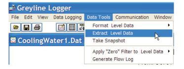
2. Select **Data Tools** from the drop down menu and then click **Generate Flow Log**. The **Channel Setup** window will open.
