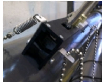
Figure 9 - Reflex Mounting Assembly - Transducer sets 'B' and 'C'
